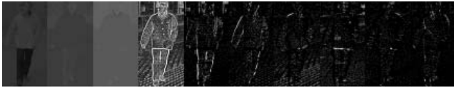
Fig. 2: Feature vector with multiple feature channels (three colour channels, pixel gradient magnitude, and gradient histograms in six angular bins) extracted from an image patch.
