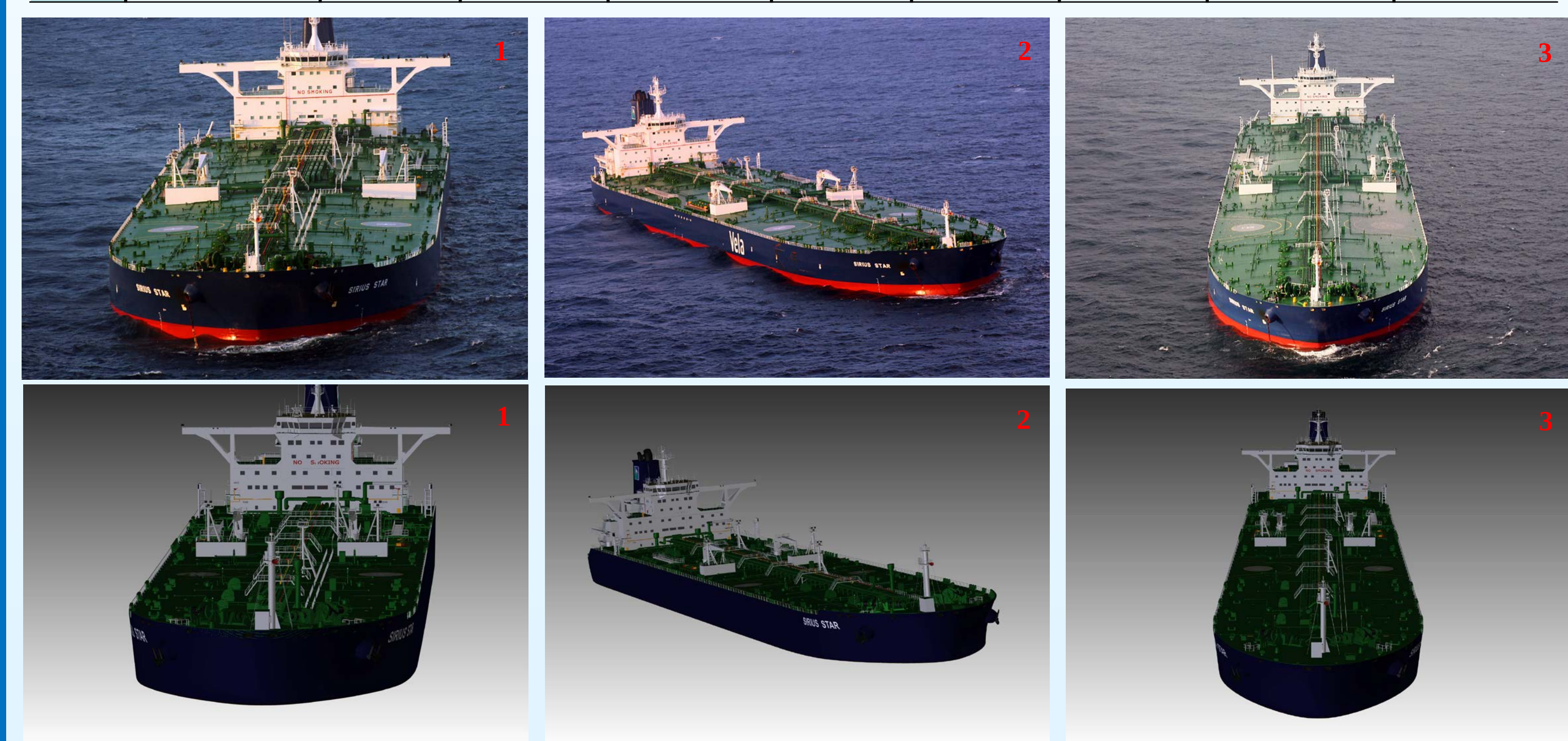
Fig.4 Photographs (upper) and rendered images (lower) of the oil tanker
