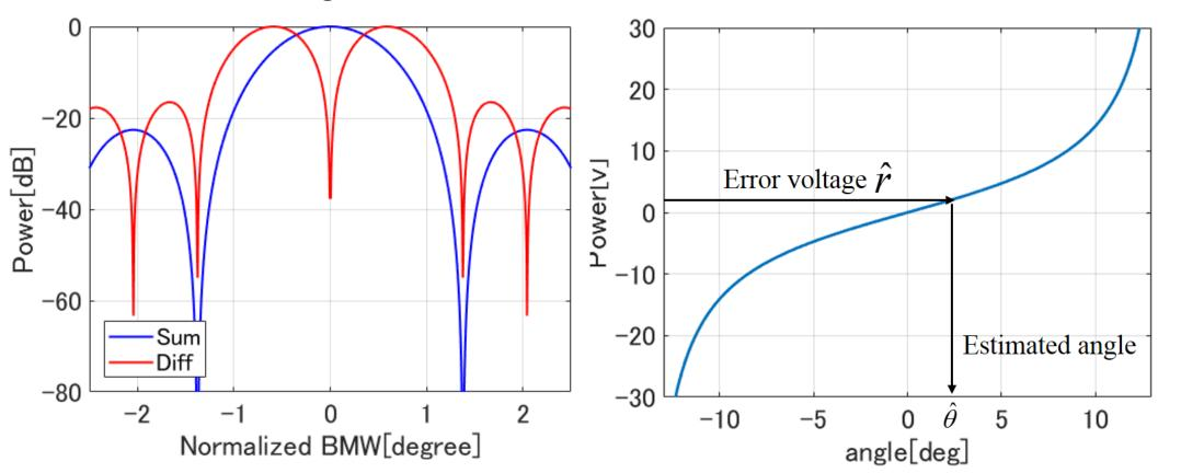
Fig. 1. Sum and difference beam pattern and monopulse ratio curve without radio interference
